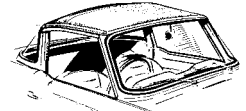
The 'Surrey Top' (a folding canopy of p.v.c.) quickly clips into position for emergency weather protection.
