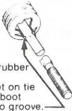
Fig. 3-3—Remove and Install Outer Tie Rod - Replaces Page 3B2-10
