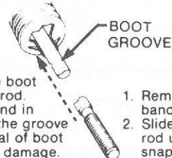
Fig. 3-3—Remove and Install Outer Tie Rod - Replaces Page 3B2-10
