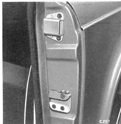
Fig. 45. Striker dovetail and door restraint
