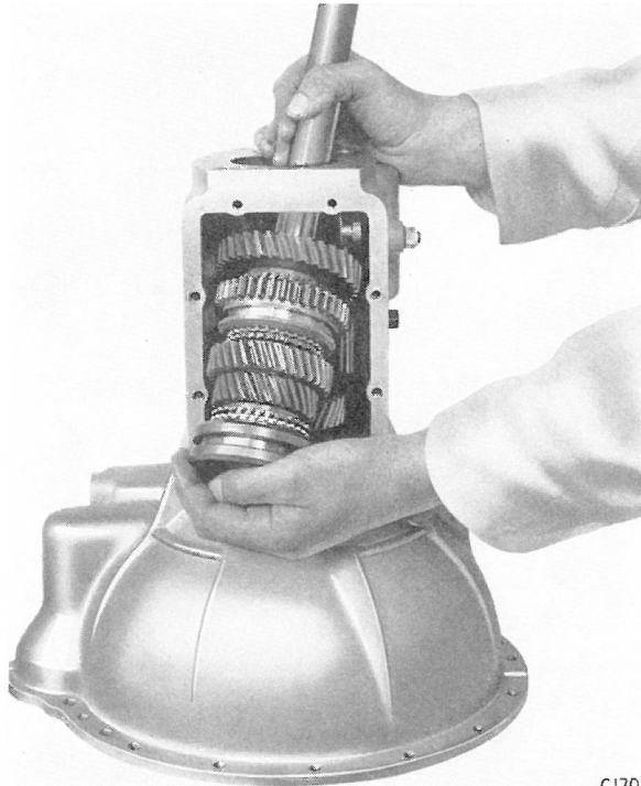
Fig. 14. Removing the mainshaft assembly
