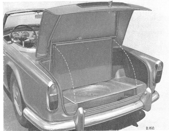
Fig. 16. Luggage locker showing hinged spare wheel cover
