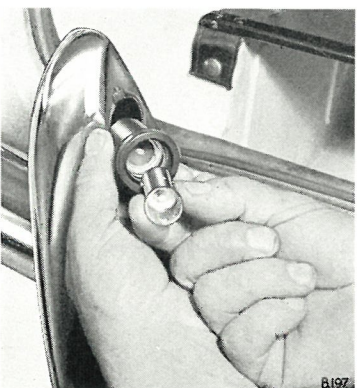
Fig. 31. Removing a bulb from plate illumination lamp
