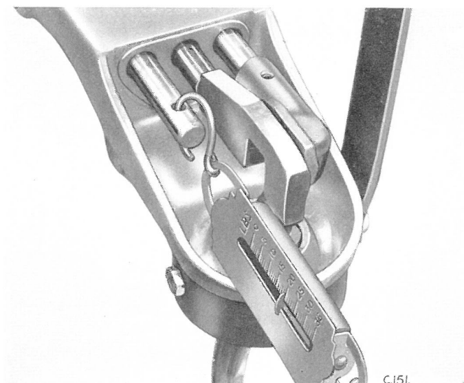
Fig. 33. Fitting a ball and spring to the 1st/2nd and 3rd/Top selector shafts. See note above.
