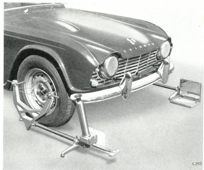
Fig. 2 Checking front wheel alignment.
