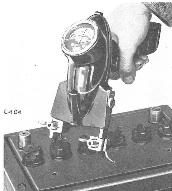
Fig. 6. Using a heavy discharge tester
