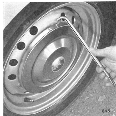
Fig. 2. Using special tool to remove nave plate from pressed steel wheel
