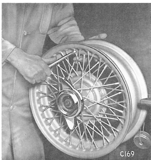
Fig. 3. Truing a wire-spoked wheel
