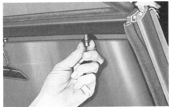
Fig. 22. Inserting screw securing roof panel to header rail
