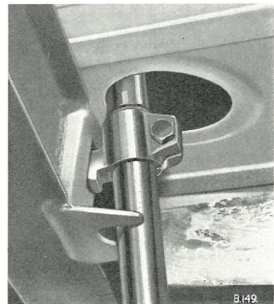
Fig. 3. The car jack located in the chassis lifting bracket
