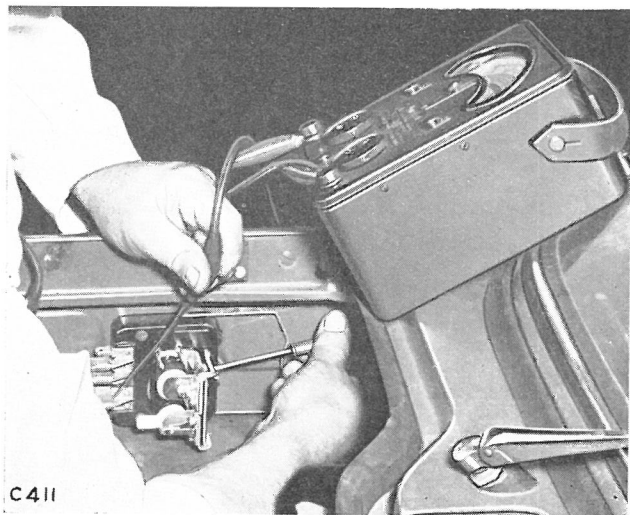
Fig. 13. Using a moving coil voltmeter to adjust the voltage regulator
