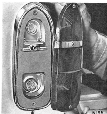
Fig. 57. Showing lens removed from stop/tail flasher lamp
