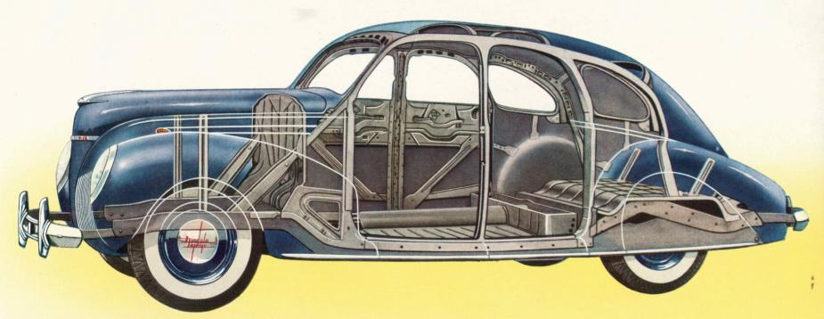
The construction of this car comes as a surprise to people used to thinking in terms of chassis and body. There is no "chassis" on the Lincoln-Zephyr—no bolted joints to squeak or rattle. Body and frame in closed types are a unit—a framework of steel trusses, in principle designed like the arch bridge, the airliner, the welded streamlined train. To this
