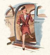
**DIRECT ENTRANCE** • You step directly from floor of car to curb. Narrow running boards are concealed and protected from dirt, ice and snow by extensions of the door panels.
