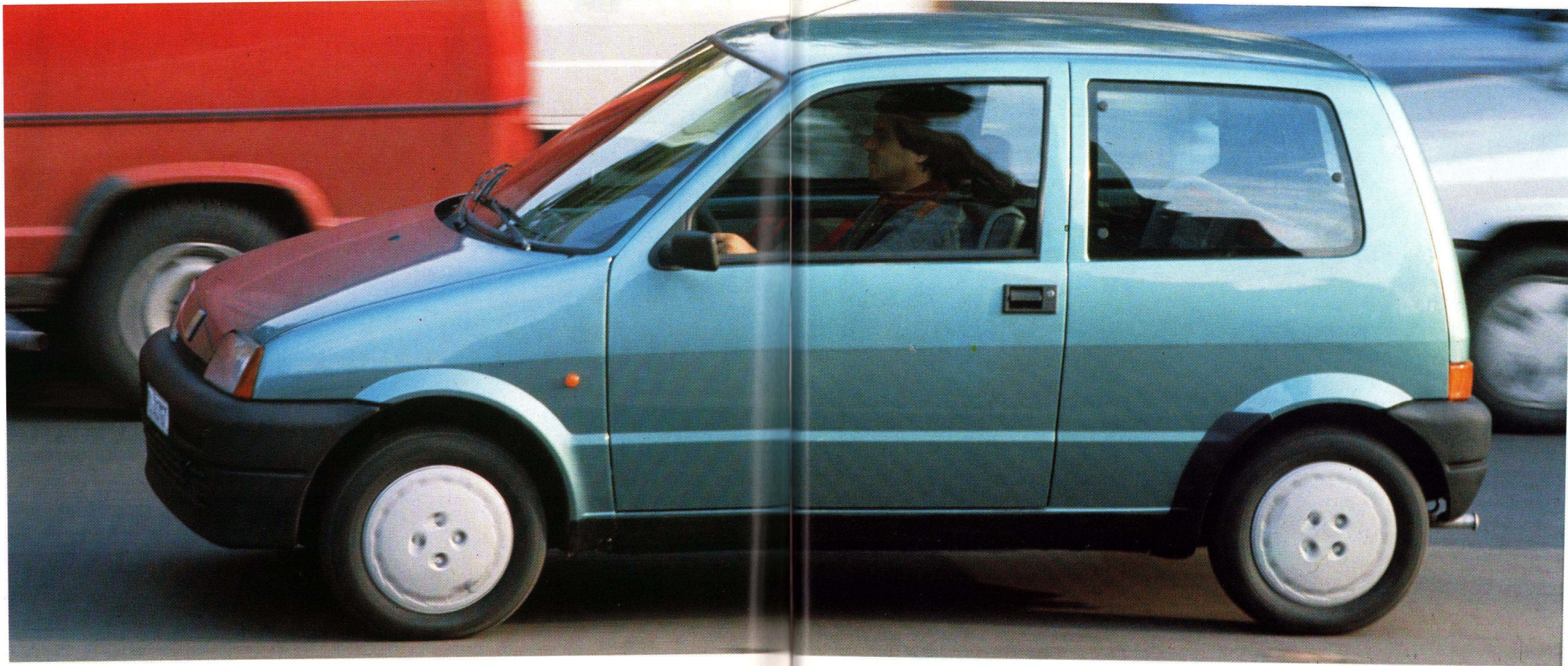
The two versions of the Cinquecento, 704 cc and 903 cc, have respective top speeds of 127 kph and 140 kph.
