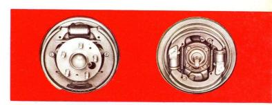
Positive action, highly efficient brakes. The front wheel brakes with two leading shoes, the rear wheel brakes with self-centering shoes and the pressure booster acting on the front wheels, ensure a progressive, symmetrical stop in the line of travel.
