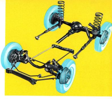
Front suspension by torsion bars and wishbones; antisway bars; double acting telescopic shock absorbers, anti-roll bar. Kingpins fitted with ball joints.
