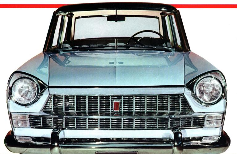
The FIAT 1800 is a 6-cylinder model, entirely new in its mechanical components and in its coachwork. It is a European class car of medium displacement. It is available with either a 1800 c.c. or a 2100 c.c. engine.
