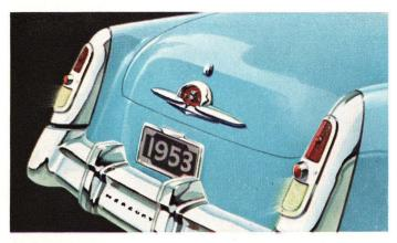
BACK-UP LIGHTS — Part of tail-lamp assembly. Go on automatically when gearshift is in reverse and lights on. Throw wide beam of light for safer backing. LOCKING GAS TANK CAP—For protecting fuel supply against theft, tampering. LICENSE PLATE FRAMES made of stainless steel with transparent plastic window.
