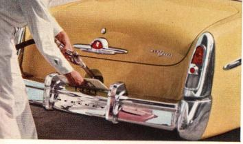
ified Design features mean extra convenience. The fill pipe for Mercury's center-fill stank is concealed behind the license plate. You can fill up from either side without pring finish. You avoid chipped finish, scratches and stains from spilled fuel.
