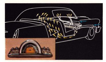
MERC-O-THERM HEATER—High-capacity hot water heater-defroster unit with 2-speed electric blower, styled exclusively for Mercury, provides comfort no matter what the weather outside. The four controls regulating heating, ventilation, and defrosting, give complete control of air temperature and its distribution.
