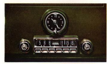
MERCURY RADIO—This superheterodyne radio with 7 tubes and rectifier is built for the acoustics of your new Mercury. Gives crystal-clear reception. Has both
