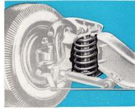
With "stedi-line" steering it takes but little On or off the pavement, on any kind of road effort to steer a Mercury—not much more than surface, Mercury's excellent front suspension finger-tip pressure. Here's another reason for gives better ride and easier handling. Steel torthe easy handling you'll enjoy in Mercury. sional stabilizer bar serves to reduce sidesway.
