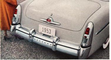
Rear bumper and rearward lights are centralized for added smartness and utility. Vertical tail-lamp fixtures house all rearward lights . . . serve as dashing bright metal fender extensions. Large bumper end caps give wrap-around protection for rear fenders.
