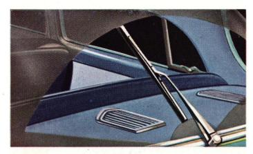
REAR WINDOW WIPER—For better rearward visibility the rear window wiper, operated by engine vacuum, whisks away snow, rain. Adds driving safety, comfort.
