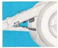
You ride cradled between the wheels in the Heavy-duty rubber bumpers for springs limit "comfort zone"-in the area of least vertical spring travel. They add to stability and smooth movement. This better ride is one of the riding. Help spring deflection rate. Provide
