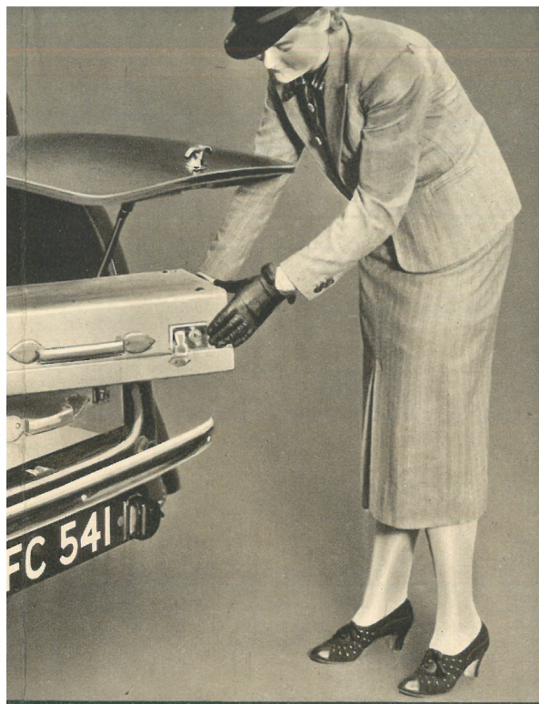
Its luggage container has external access by means of a door. Capacity of the container is nearly 5½ cubic feet.
