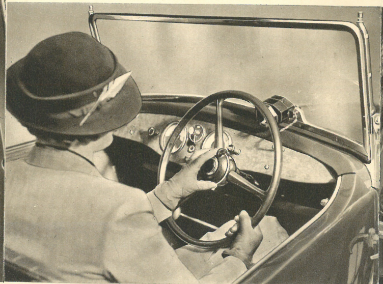
The driving position is exceptionally comfortable and wheel centre control is provided for the self-cancelling trafficators and electric horn. The instrument panel on the open model is neat and practical.
