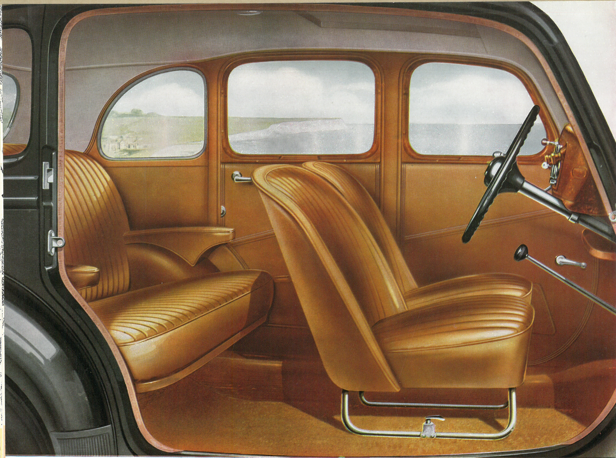
The interior accommodation of the Morris Ten-Four (Series "M") is particularly spacious. The rear seat has an elbow width of 51 in. and the front seats are of the metal framed type with floating spring seat base and flush-type runners for adjustment.
