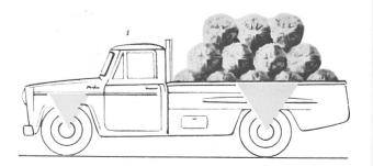
Balanced weight distribution on front and rear wheels provides good road holding qualities and riding comfort with any loads.
