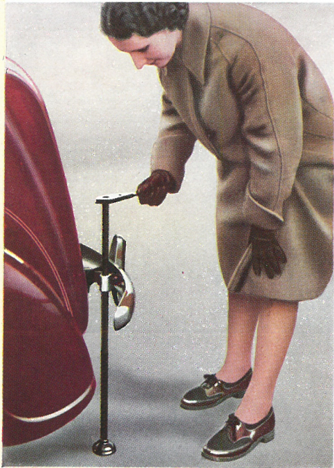
Jacking. —The simple but easy and efficient jacking system.
