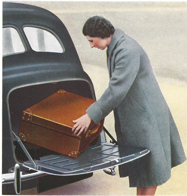
Luggage. —The large built-in luggage compartment with spare wheel. The hinged panel accommodates extra suitcases.
