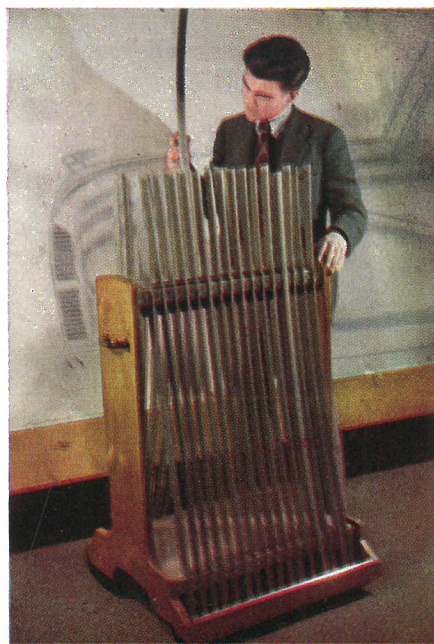
Sweeps, or standard curves, enable each element of the body line to be precisely specified by number.
