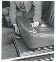
Wide, divided, benchtype front seats are independently adjustable on slides to suit the individual needs of driver and passenger. Each seat has a fore and aft movement of 5 in.
