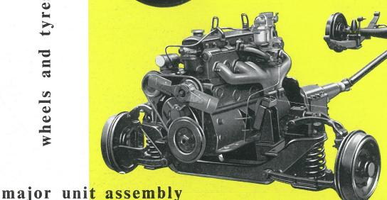
Due to the fact that the coachwork of the Westminster is of unitary construction, all the major mechanical units are assembled as one before being mounted to the body.
