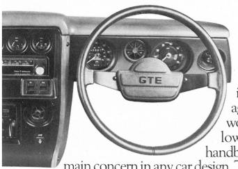
immediate reach and the fascia incorporates special early warning instrumentation against failed brakes, worn brake pads, low fuel and engaged handbrake. Safety is a
