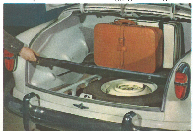
the spare wheel, situated under the luggage compartment floor, enables maximum use to be made of the space available for luggage storing
