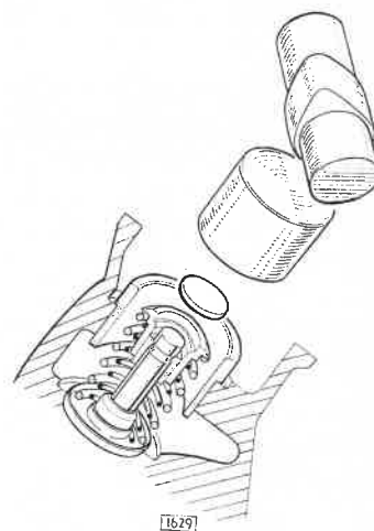
Fig. 73. The pad for adjustment of the valve clearance is situated between the tappet and the top of the valve stem.
