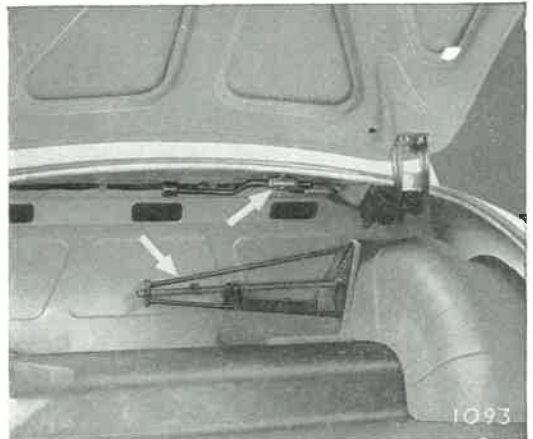
Fig. 8. The wheel brace and jack are retained in clips at the front of the luggage compartment. The jack handle is stored in the tool container.
