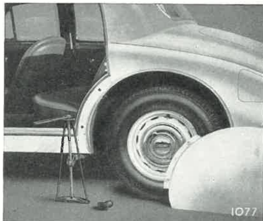
Fig. 12. The jack in position for raising the left-hand rear wheel.
