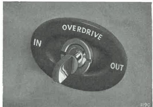
Fig. 9. Overdrive control switch.
