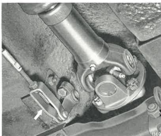
Fig. 52. Handbrake cable adjustment.
