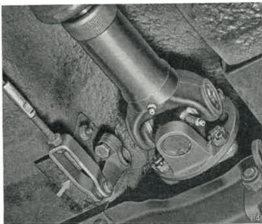
Fig. 28. Handbrake cable adjustment.
